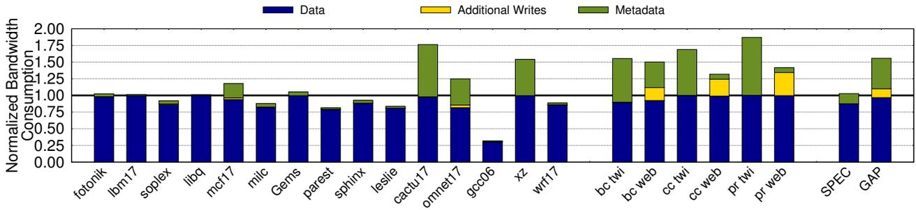
Fig. 4. Bandwidth consumption for data, additional writes to compress data, and metadata for TMC design with table-based metadata, normalized to uncompressed memory. Metadata accesses incur significant bandwidth overhead.
