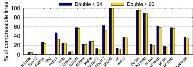
Fig. 6. Probability of a pair of adjacent lines compressing to  $\leq 64B$  and  $\leq 60B$ . We can use 4B to store metadata, without significantly affecting compressibility.
