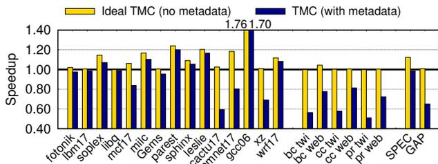
Fig. 5. Speedup from ideal TMC (no metadata lookup) and TMC with metadata (w/ metadata cache), relative to uncompressed memory.
