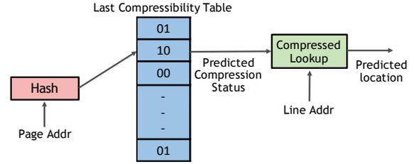
Fig. 8. Line Location Predictor uses line address and compressibility-prediction (based on last-time compressibility) to predict location.
