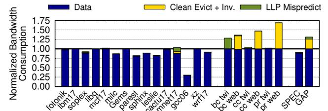
Fig. 14. Bandwidth consumption for PTMC approach, normalized to uncompressed memory.
