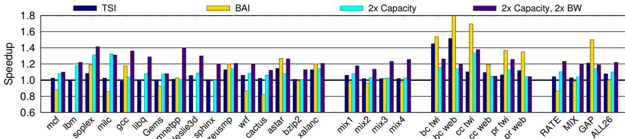
**Figure 7: Speedup from Traditional Set Indexing and Bandwidth-Aware Indexing, compared to doubling the cache capacity and bandwidth. BAI improves bandwidth for compressible workloads but causes slowdown for others due to thrashing.**
