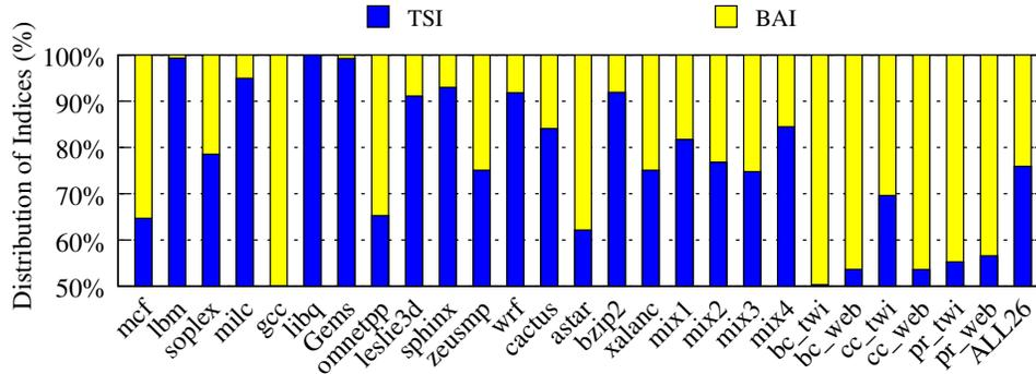
**Figure 11: Distribution of BAI and TSI for a cache compressed with DICE. Note that for 50% of accesses, we do not need to make install decisions or do index prediction as TSI and BAI refer to the same set, hence the y-axis starts at 50%.**
