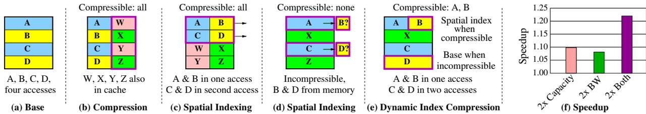
**Figure 1: Considerations in compressing DRAM caches (a) Baseline system with four lines (A-D) (b) Compression for capacity (c) Spatial indexing for bandwidth (d) Slowdown from spatial indexing when data is incompressible (e) Dynamic index compression based on compressibility (A, B use spatial index) (f) Potential speedup from doubling DRAM cache capacity, bandwidth, and both.**
